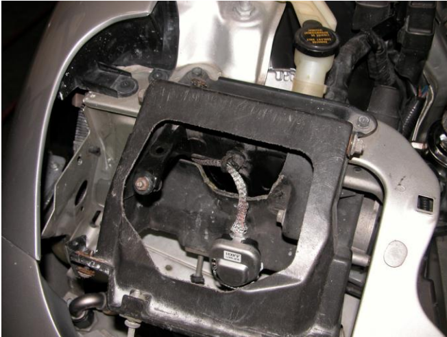
5. Routing of the bulb connector on our prototype kit (we re-used the factory cable holder)
