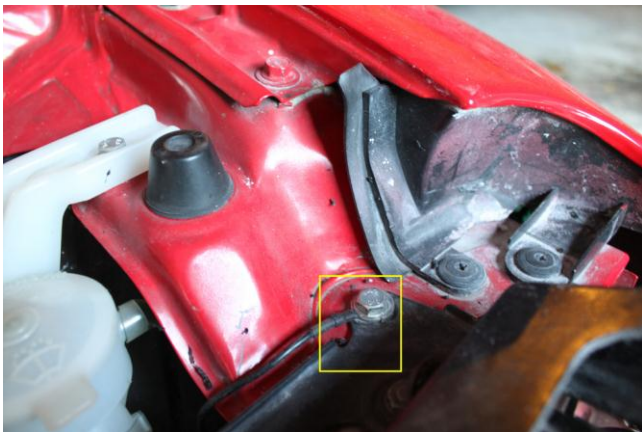
4. Example of a grounding point. You can use any suitable grounding point.
