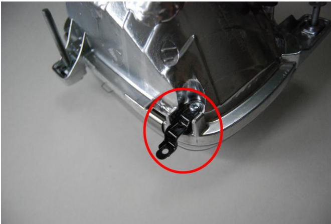
7. Pull spring with pliers to attach to stabilizer foot
